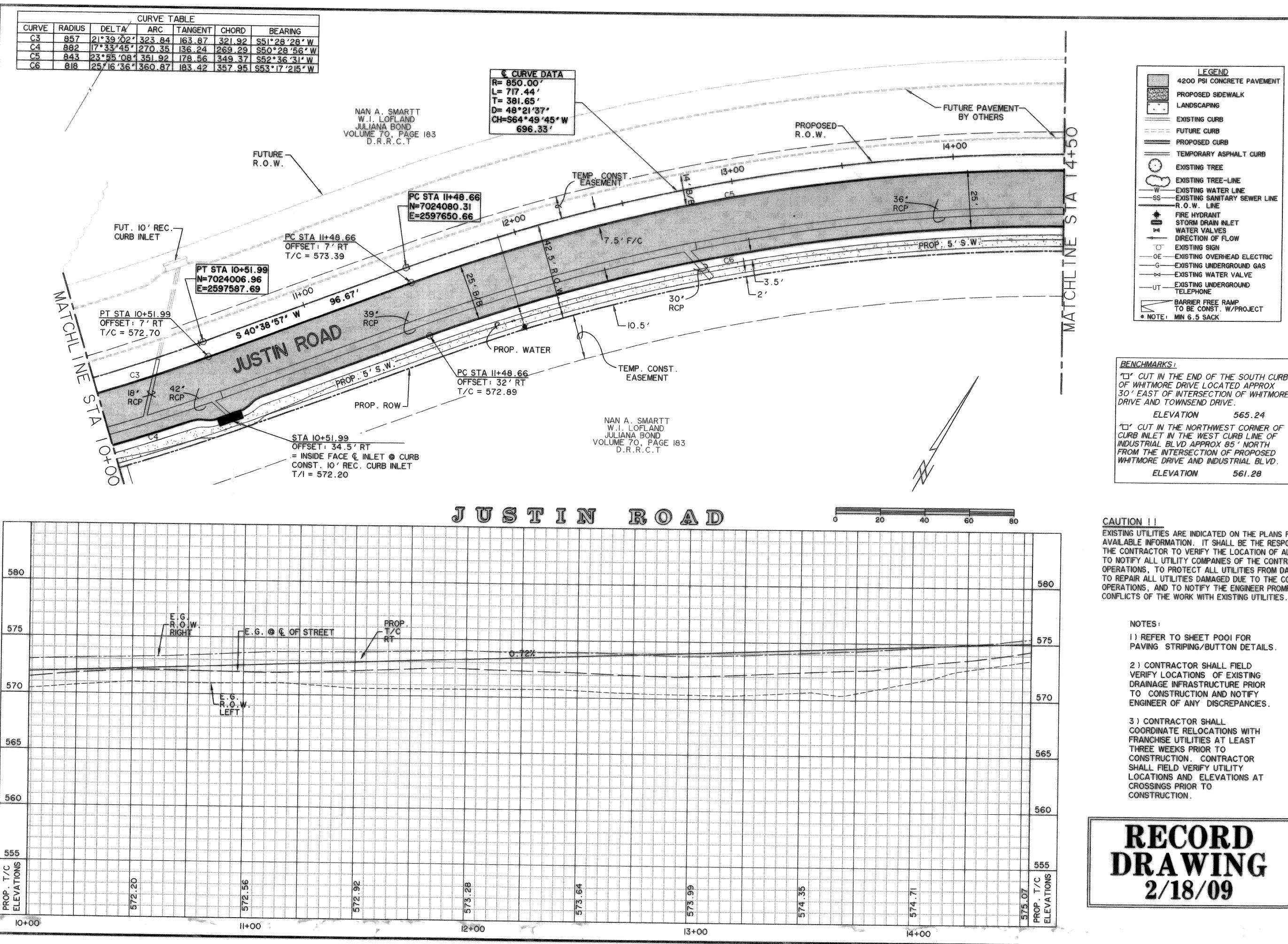
LEGEND 4200 PSI CONCRETE PAVEMENT PROPOSED SIDEWALK LANDSCAPING **EXISTING CURB** === FUTURE CURB PROPOSED CURB TEMPORARY ASPHALT CURB EXISTING TREE >>> EXISTING TREE-LINE -W---EXISTING WATER LINE -SS---EXISTING SANITARY SEWER LINE -R.O.W. LINE FIRE HYDRANT STORM DRAIN INLET WATER VALVES DIRECTION OF FLOW TO EXISTING SIGN OE -EXISTING OVERHEAD ELECTRIC ----G-EXISTING UNDERGROUND GAS ------EXISTING WATER VALVE \_\_EXISTING UNDERGROUND TELEPHONE
