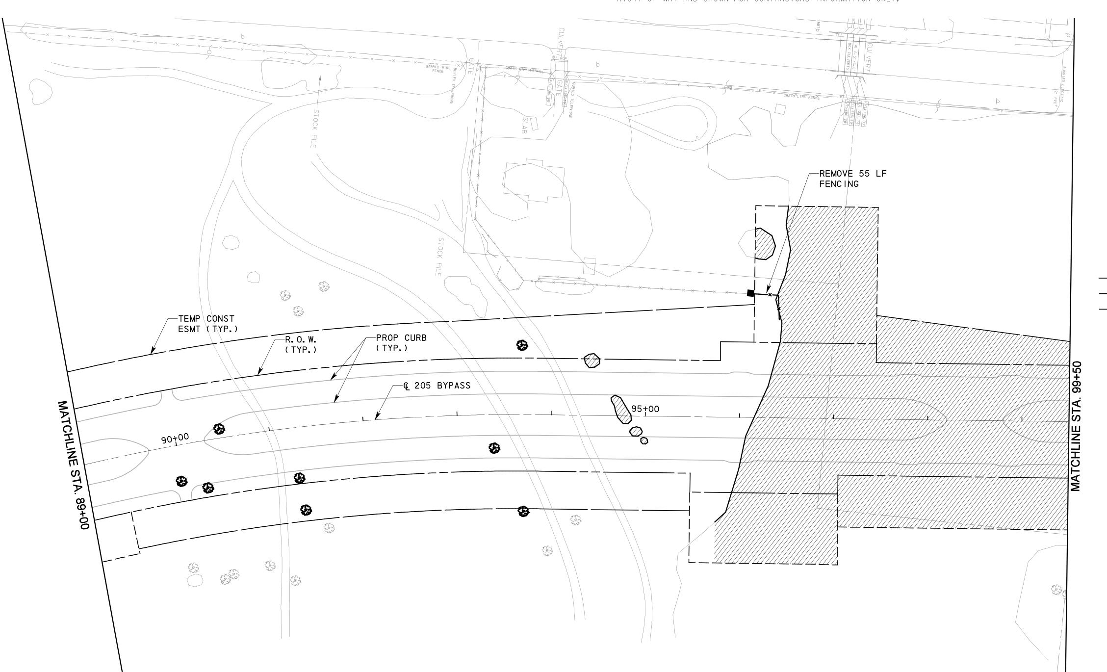
EXIST. TREE TO REMAIN EXIST. FENCE TO REMAIN EXIST. TREE TO BE REMOVED (SEE NOTE 3) EXIST. FENCE TO BE REMOVED EXIST. BRUSH & SMALL DIAMETER TREES TO BE REMOVED EXIST. ASPHALT PAVEMENT TO BE REMOVED EXIST. CONCRETE TO BE REMOVED PROP FENCE CORNER/PULL POST (MATCH EXIST FENCE TYPE PER TXDOT DETAIL WF(I)-94 OR WF(2)-96) PROPOSED RIGHT-OF-WAY DRAINAGE EASEMENT TEMP. CONSTRUCTION EASEMENT
