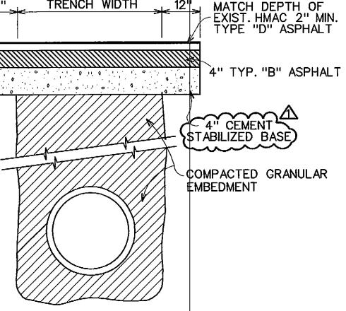
ASPHALT PAVING REPLACEMENT (FOR ALL TYPES OF PIPES)
