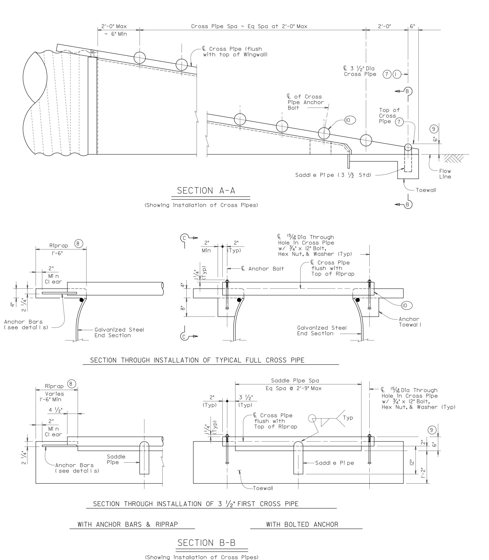
Size and Lengths of Cross Pipes shallbe as shown in the tables, except the first Cross Pipe from the bottom and the associated Saddle Pipe shallbe 3 1/2". All other values shown are minimum requirements.
