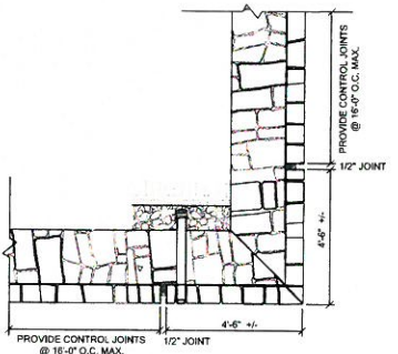
RW1/4 TYPICAL PLAN VIEW AT CORNER SCALE: N.T.S.
